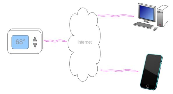
The system shall consist of three tiers: embedded system, web service, and client applications.
